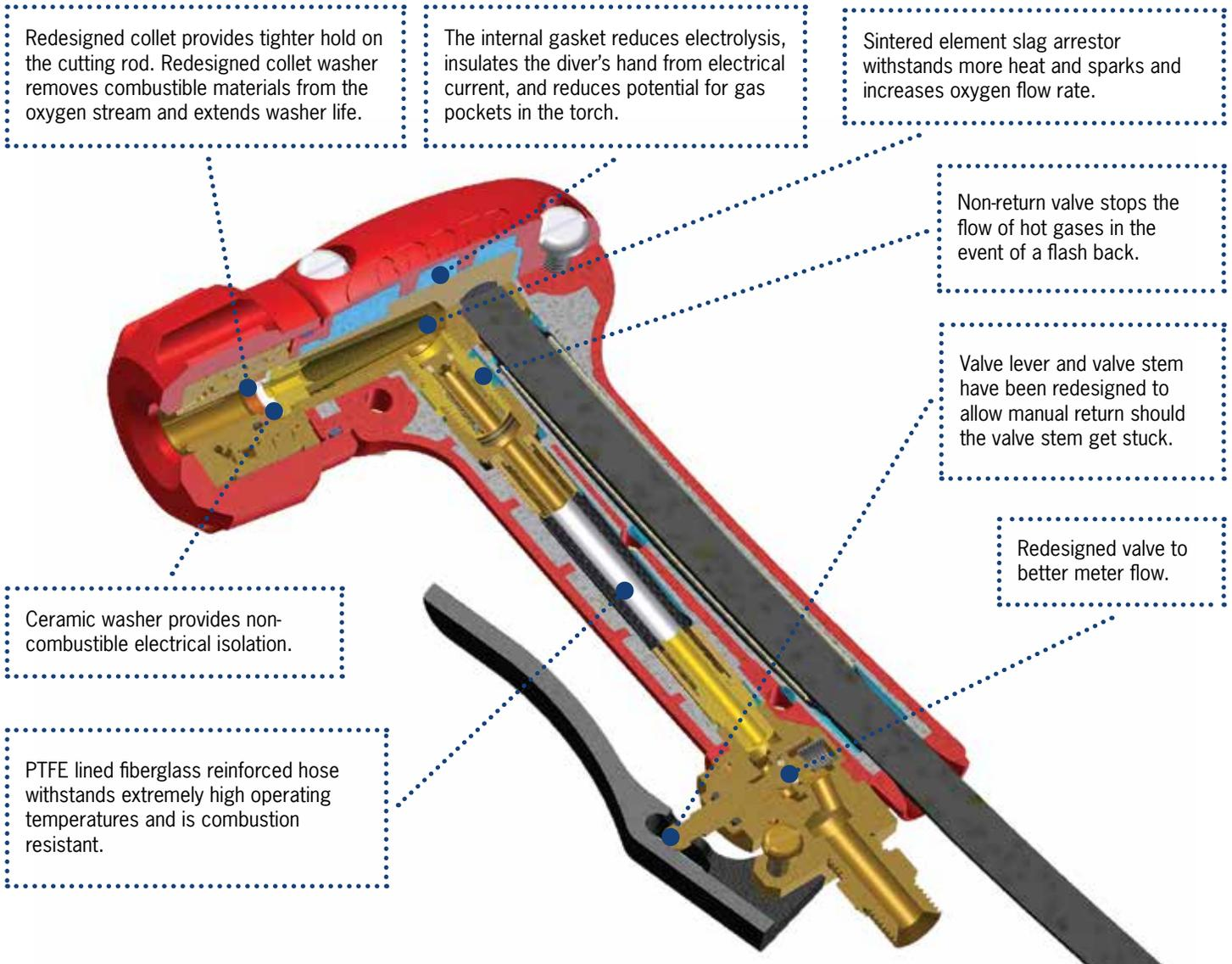
Redesigned collet provides tighter hold on the cutting rod. Redesigned collet washer removes combustible materials from the oxygen stream and extends washer life.
