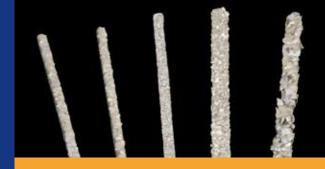
**PMA Diamond Carbide Hardfacing Rods** are a special blend of tungsten carbide sintered with nickel, chromium, and boron powder. The nickel alloy matrix offers the ultimate in extreme wear protection, and has a lower melting point than iron-based products. Tungsten carbide is available in multiple sizes to address usage needs.
