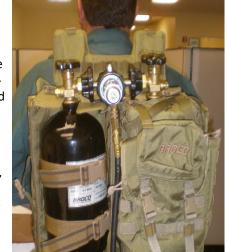
PC/TACMOD1 includes a 12V gel cell battery that is used with the striker plate to quickly and easily ignite standard Broco cutting rods. An oxygen transfill hose assembly, cutting rod extension, and Broco's SNAP quick-connect cutting rod system also come in the set.
